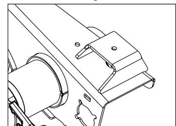
With 2-inch, weld-on air spring pedestal
