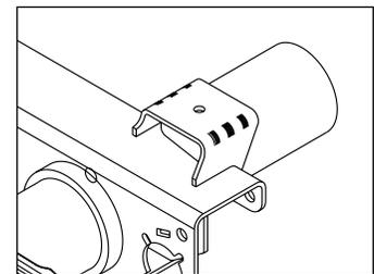
With weld-on air spring pedestal
