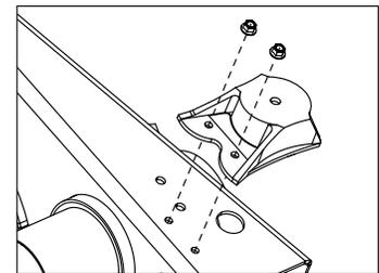
With cast, bolt-on air spring pedestal
